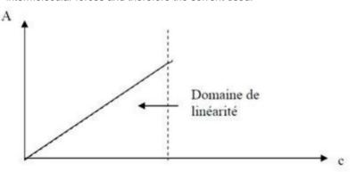
The graph representing absorbance as a function of concentration, called a **calibration** line (or **curve**), allows the unknown concentration of of a solution to be determined from the measurement of spectrophotometric absorbance.
