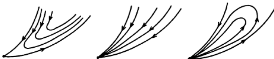
Figure 1. (a) A hyperbolic sector. (b) A parabolic sector. (c) An elliptic sector.
