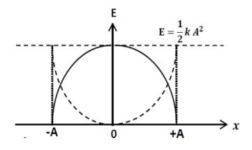
Fig.12. Variation of kinetic, potential and total energies as a function of x
