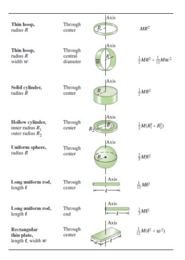
Fig.10. inertia of different shapes
