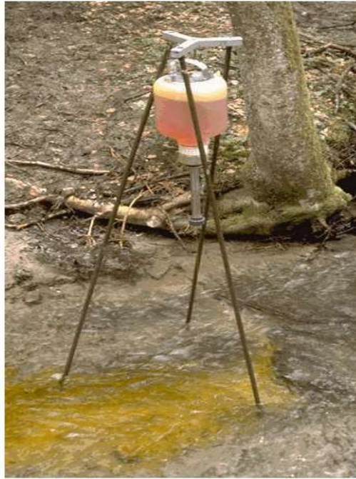
Fig. Constant flow gauging.
