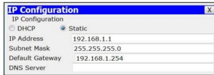
The gateway for this network is the Fa 0/1 interface of the router, with the address 192.168.1.254
