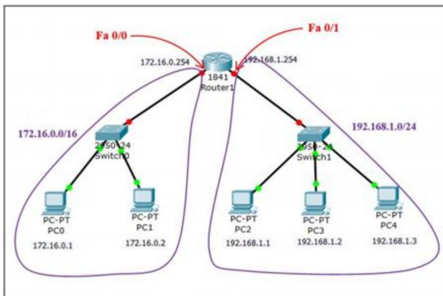
This network consists of two local networks: LAN1 with IP 172.16.0.0 and LAN2 with IP 192.168.1.0. Both networks are connected via a router. LAN1 is connected through the FastEthernet 0/0 interface (denoted as Fa 0/0) and LAN2 through the FastEthernet 0/1 interface (denoted as Fa 0/1).
