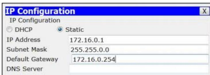
The gateway for this network is the Fa 0/0 interface of the router, with the address 172.16.0.254. Do the same for the other PCs in this network.
