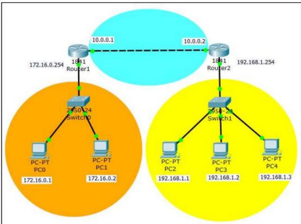
The router interfaces are configured, taking into account this time the addition of a third LAN network.
