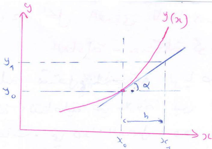
$$\text{tg}(\alpha) = \frac{y_1 - y_0}{h} \Rightarrow y_1 - y_0 = h \text{tg}(\alpha) \quad / \quad \text{tg}(\alpha) = y'(x_0) = f(x_0, y_0)$$
