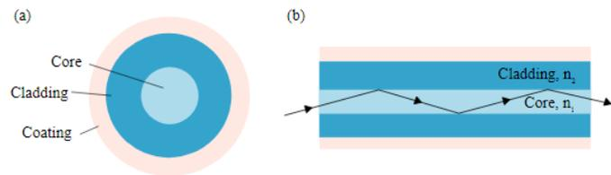
(a) Diagram of a bare fiber in the surrounding. (b) propagation of light by total internal reflection inside of an optical fiber.
