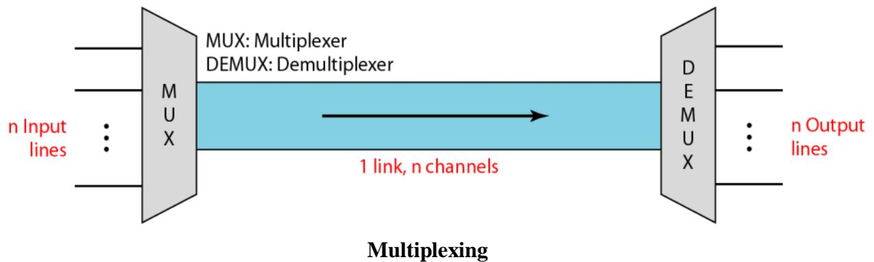
A multiplexer takes several inputs, which are transmitted over a high capacity signal link. At the receiving end, the demultiplexer separates the data and delivers it to appropriate output line.
