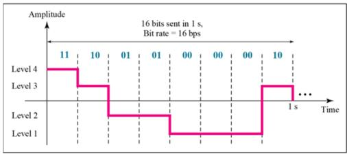
b. A digital signal with four levels
