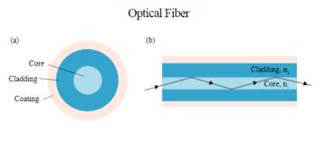
(a) Diagram of a bare fiber in the surrounding. (b) propagation of light by total internal reflection inside of an optical fiber.
