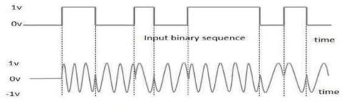
BPSK Modulated output wave
