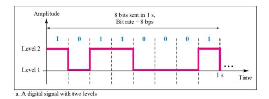
Since a digital signal can have many discrete levels, more than one bit can be transmitted for each level. If a digital signal has **L** levels, the number of bits each level represents can be calculated as:
