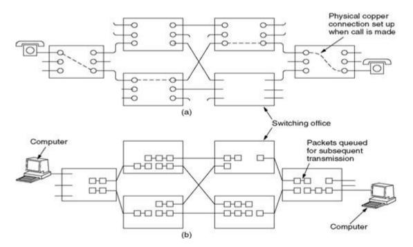
Here, the six rectangles represent switching offices, each having 3 incoming and 3 outgoing lines. When a call is placed, a physical connection is established between the incoming line and one of the output lines (shown by dotted lines).
