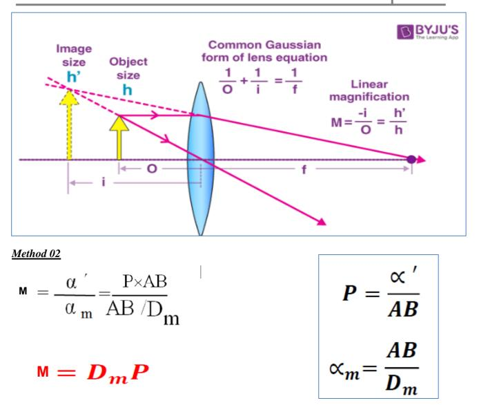
*The magnification* of a microscope is equal to the product of its power by the minimum distance (**Dm**) of distinct vision of the eye using it.
