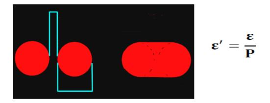
The resolving power of an <u>objective lens</u> is measured by its ability to differentiate two lines or points in an object. The greater the resolving power, the smaller the minimum distance between two lines or points that can still be distinguished. The larger the <u>N.A.</u>, the higher the resolving power.
