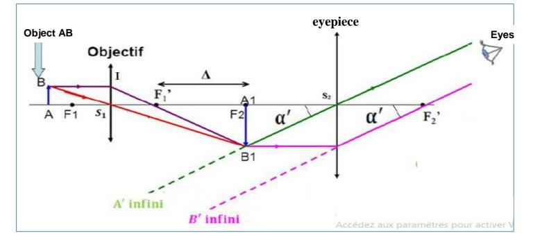
$$\gamma_{obj} = \frac{\overline{A_1 B_1}}{\overline{AB}} = \frac{\overline{A_1 B_1}}{\overline{S_1 I}} = \frac{\overline{F_1' F_2}}{\overline{F_1' S_1}} = \frac{\Delta}{f_1'}$$
