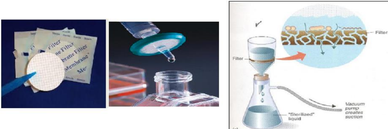
Figure 4: Liquide filtration using membrane filtration
