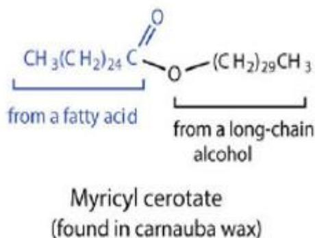
Figure 9: Structures of Wax.
