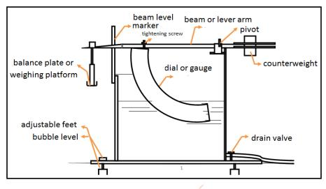
Figure 1. Experimental device
