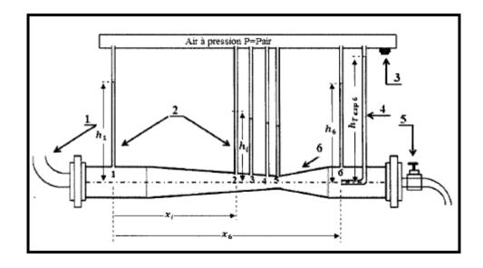
Figure.IV.2. Flow in a convergent-divergent.
