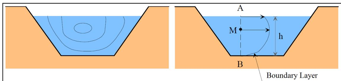
Figure.V.3.Velocity Distribution in a Straight Section of a Channel
