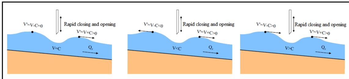
**Figure.V.2.** Creation of Disturbance in an Open Channel.
