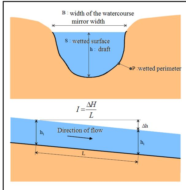
**Figure V.1.** Flow in an Open Channel.
