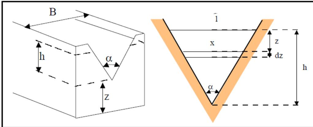
**Figure.V.7.**Triangular Thin-Plate Weir.
