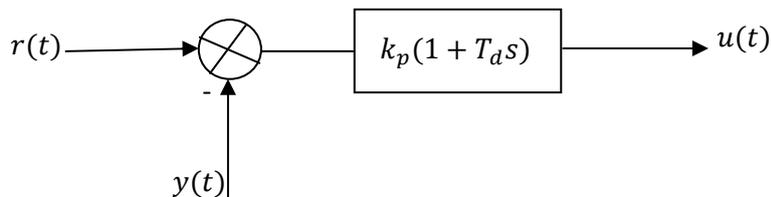
$$u(t) = k_p \left( e(t) + T_d \frac{de(t)}{dt} \right) \Rightarrow C(s) = \frac{U(s)}{E(s)} = k_p(1 + T_d s)$$
