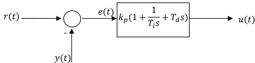
$$u(t) = k_p(e(t) + \frac{1}{T_i} \int_0^t e(\tau) d\tau + T_D \frac{de(t)}{dt}) \Rightarrow C(s) = \frac{u(s)}{e(s)} = k_p(1 + \frac{1}{T_i s} + T_D s)$$
