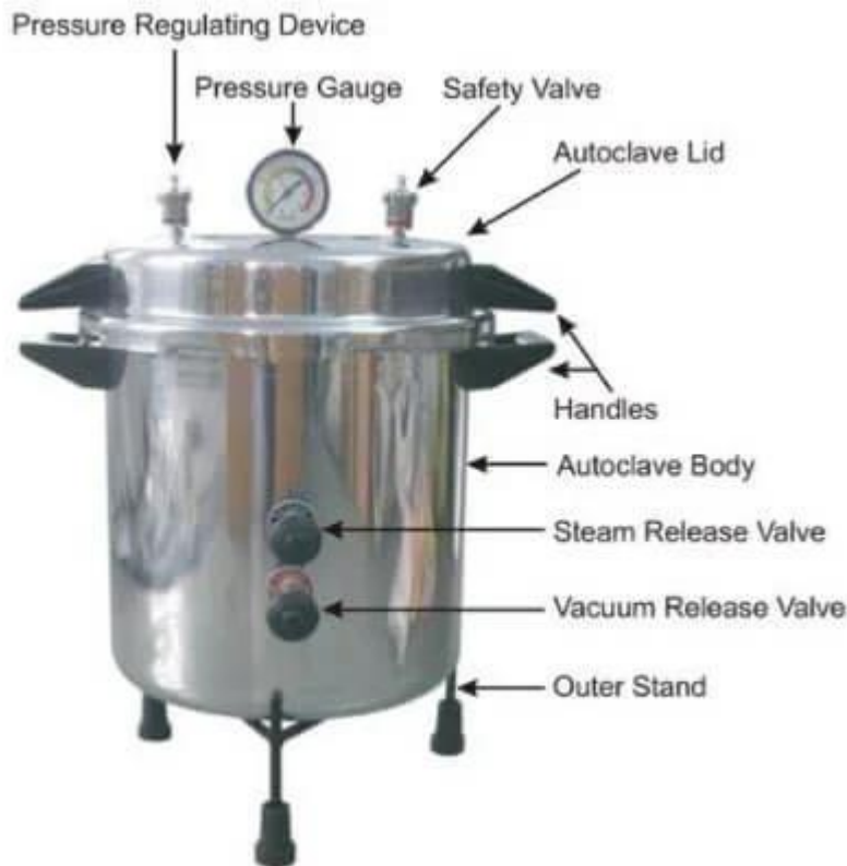
Fig 2: A schematic diagram of autoclaves with their different labeled parts.
