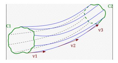
**Trajectory:** It is the curve described over time by a fluid particle, i.e. each fluid particle that we follow in its movement (Lagrangian description) describes a trajectory that we determine by solving the following equation:
