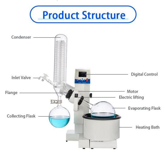
Fig 1: structure of Rotovap https://www.laboao.com/
