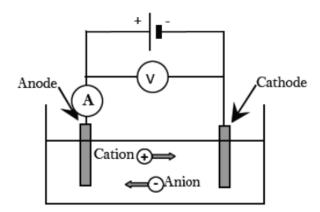
Figure 1: Representative diagram of the principle of electrical conduction in electrolytic solutions.
