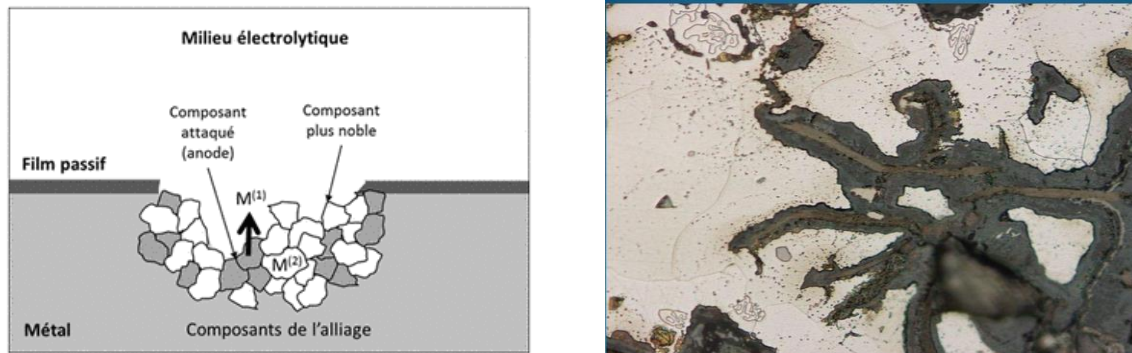
Fig.13. Selective Corrosion on cast iron
