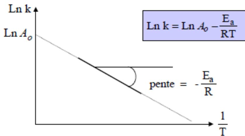
$$\text{à } T_1: \text{Ln } k_1 = \text{Ln } A_0 - \frac{E_a}{RT_1} \quad (1)$$
