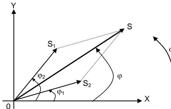
$$S(t) = S_1(t) + S_2(t) = S \cdot \sqrt{2} \sin(\omega t + \varphi)$$
