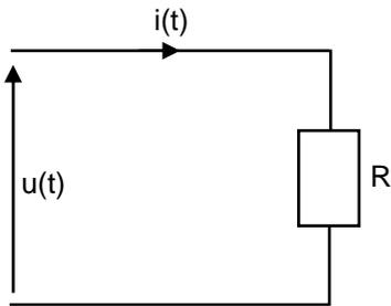
$$u(t) = U\sqrt{2} \sin(\omega t + \varphi_0) \Rightarrow i(t) = I\sqrt{2} \sin(\omega t + \varphi_1)$$
