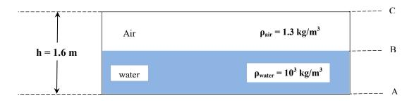
1- Calculate the pressure difference between points **A** and **B**.
