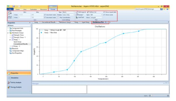
To compare data from more than one crude assay, the second crude must be added, you can add it to the plot by clicking "Select Assays" under the Format tab when the Plot is selected.
