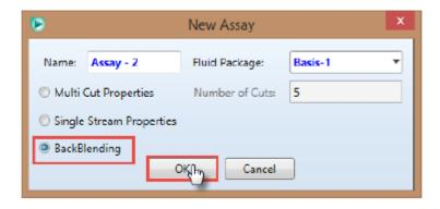
After selecting Backblending, the Backblending Input Form appears on the navigation pane instead of the Input Assay Form.
