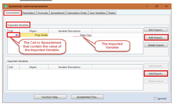
You can import virtually any variable in the simulation into the Spreadsheet, and you can export a cell's value to any specifiable field in your simulation.
