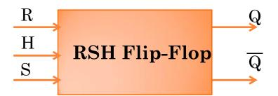
The RSH flip-flop is a: synchronized RS flip-flop with a clock signal H.
