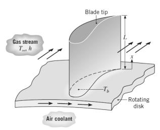
The blades, which are fabricated from Inconel,  $\mathbf{k} \approx 20 \text{ W/m·K}$ , have a length of L = 50 mm. The blade profile has a uniform cross-sectional area of  $A_c = 6 \times 10^{-4} \text{ m}^2$  and a perimeter of P = 110 mm. A proposed blade cooling scheme, which involves routing air through the supporting disc, is able to maintain the base of each blade at a temperature of  $T_b = 300^{\circ}C$ .
