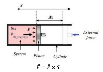
When an external operator exerts a force on the piston, it moves to the left: the gas then exerts a force 'F'; Where: 'F' is in Newton (N); 'S' is in square meter (m<sup>2</sup>).
