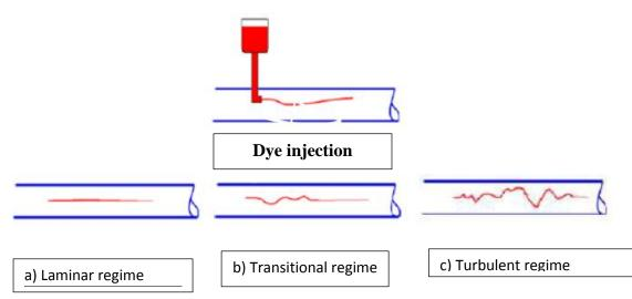
By using various fluids (different viscosity), varying the flow rate and diameter of the pipeline, Reynolds showed that the parameter which made it possible to determine whether flow is laminar or turbulent is a dimensionless number called the number of Reynolds . It expresses the relationship between the inertia force.  $\rho\mu$  and the viscous force  $\mu * \frac{u}{d}$
