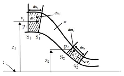
At t time : the fluid between S1 and S2 has a mass equal to dm+mAt instant t+ dt the fluid between S1 ' and S2' to a mass equal to (m + dm2)By conservation of mass:
