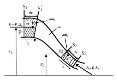
Let us apply the kinetic energy theorem to (The variation of kinetic energy is equal to the sum of the work of external forces
