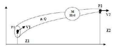
When fluid passes through a hydraulic machine, it exchanges energy with this machine in the form of work  $\Delta W$  for a duration  $\Delta t$ . The power P exchanged is:
