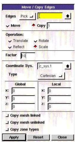
Select the front cylinder edge. Make sure that the *Copy* is checked. Under *Operation*, select *Scale*. Next to *Factor*, enter a value of 10. This means that the radius of influence we create will be 10 times the size of the cylinder. Click *Apply*.
