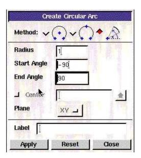
Next to *Radius*, enter 1. Next to *Start Angle*, enter -90. Next to *End Angle*, enter 90. Click *Apply*. Do the same for front arc but enter different value for angles.
