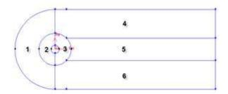
We set the geometry upstream to be shorter because we have less activity before flow through cylinder. We set the geometry downstream of the cylinder to be relatively longer such that the boundary conditions will not affect the flow near cylinder.
