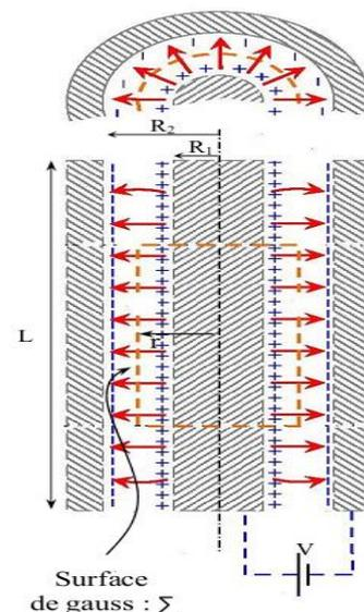
$$\vec{E} = \text{grad}V \Rightarrow E = -\frac{dV}{dr} \Rightarrow dV = -\vec{E} \cdot d\vec{r} = -E \cdot dr = \int_1^2 -dV = \int_{R_1}^{R_2} \frac{Q}{2\pi r L \epsilon_0} dr \Rightarrow V_1 - V_2 = \frac{Q}{2\pi L \epsilon_0} \log \frac{R_2}{R_1}$$
