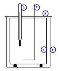
Figure 1. The calorimeter
