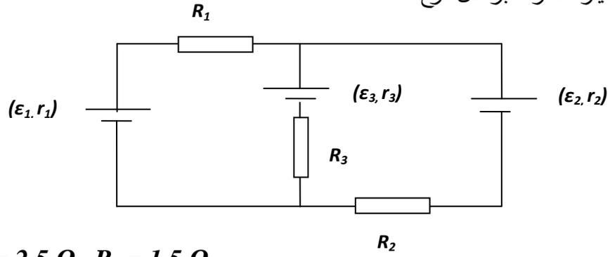
$$R_1 = 1.5 \Omega \quad R_2 = 2.5 \Omega \quad R_3 = 1.5 \Omega$$
