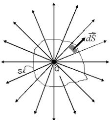
$$\phi = \iint_S \vec{E} \cdot \vec{ds} = \iint_S \frac{kQ}{r^2} \vec{u} \cdot \vec{ds} = kQ \iint_S \frac{\vec{u} \cdot \vec{ds}}{r^2} = kQ \iint_S d\Omega = kQ(\Omega) \quad \text{البرهان:}$$
